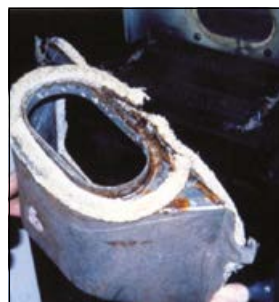
Some examples of rope seals found on boilers
