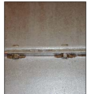
String gasket between metal sheets
