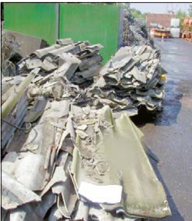
Asbestos waste discarded illegally
