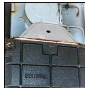
String gasket between metal sheets
